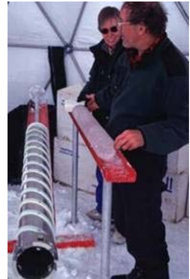
Here researchers are pulling a core of ice that they extracted from a glacier in the Andes Mountains of South America. In the right picture, you can see the hollow drill that was screwed downward into the glacier. The ice core came out of the pipe. Photos courtesy Lonnie Thompson, Ohio State University.
