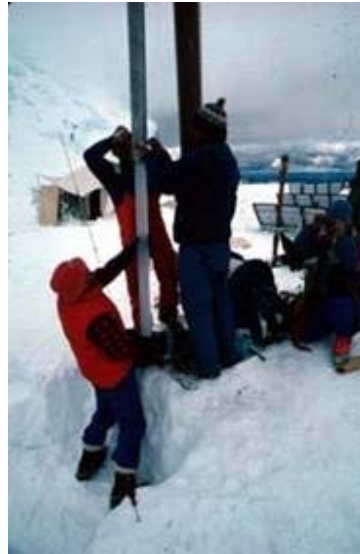
Here researchers are pulling a core of ice that they extracted from a glacier in the Andes Mountains of South America. In the right picture, you can see the hollow drill that was screwed downward into the glacier. The ice core came out of the pipe. Photos courtesy Lonnie Thompson, Ohio State University.
