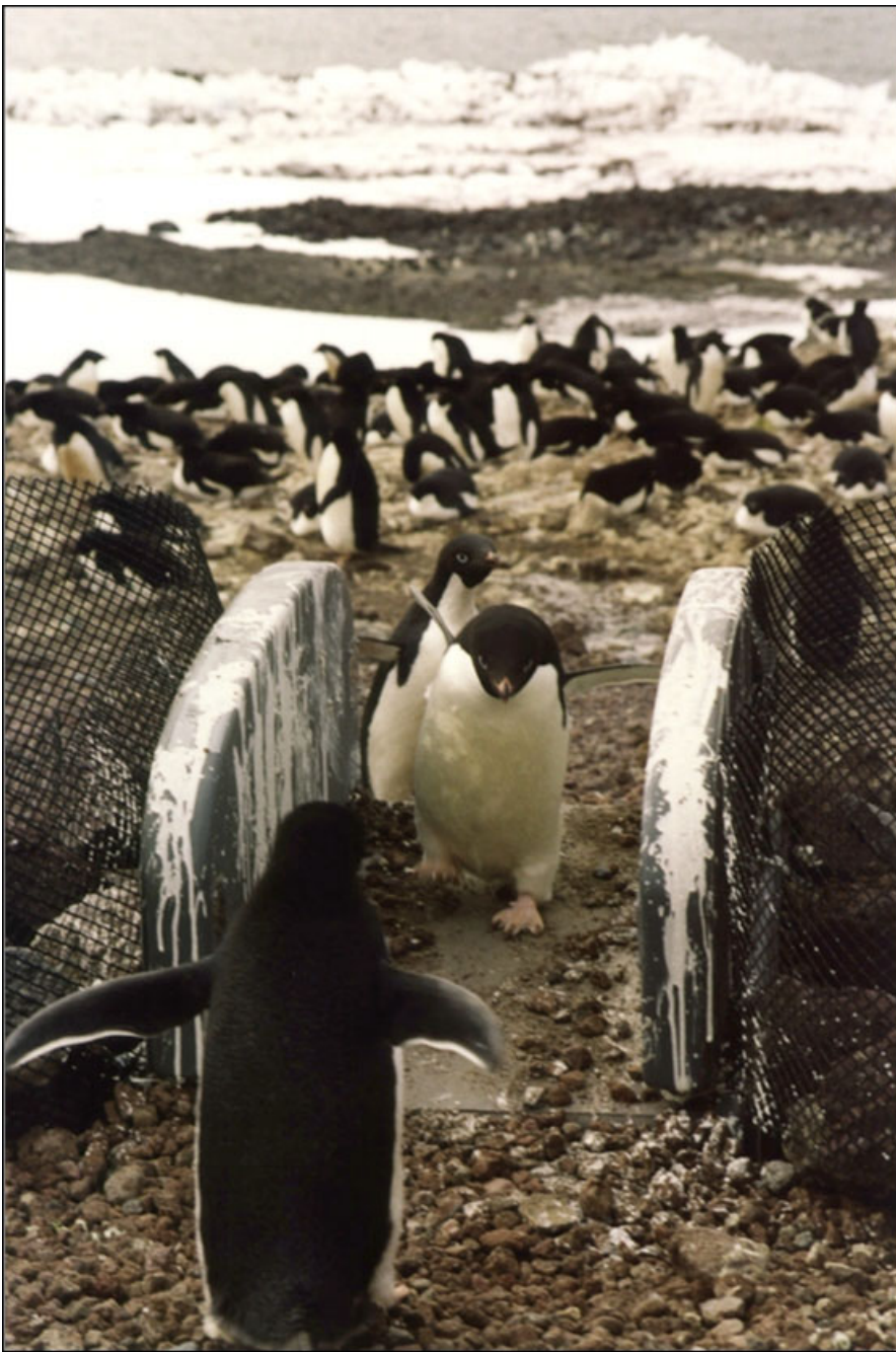
Corridor weighbridge works, but RFID performance is marginal Source: Beigel Technology Corp
